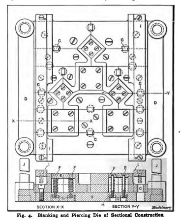
sections are machined approximately to the required dimensions with the exception of the inside or cutting edges, which were left a few thousandths over size to permit grinding them after hardening. The face is recessed on the outer edge to within  $\frac{1}{4}$  inch of the cutting edge and  $\frac{5}{8}$  inch from the bottom, thus
